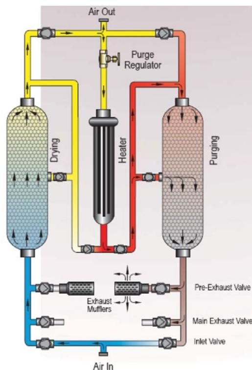
**FIGURE 6.** Externally heated desiccant dryer flow path
