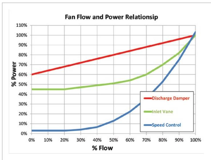
**FIGURE 9.** Sample part-load performance of various fan control methods
