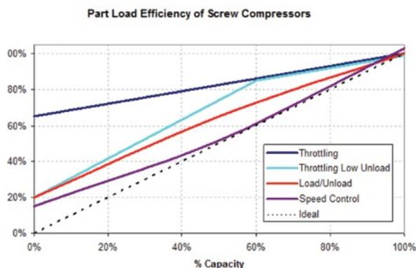
**FIGURE 2.** Sample part-load performance of oil injected screw air compressors
