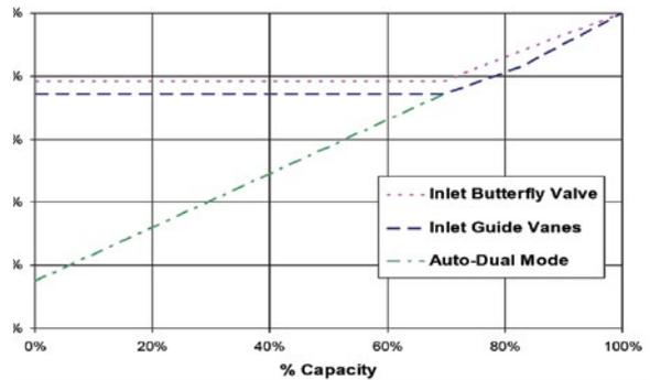
FIGURE 4. Part load control methods of centrifugal compressors
