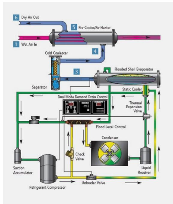
FIGURE 5. Refrigerated dryer flow path
