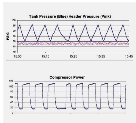
**FIGURE 3.** Load/unload cycle pressure and power
